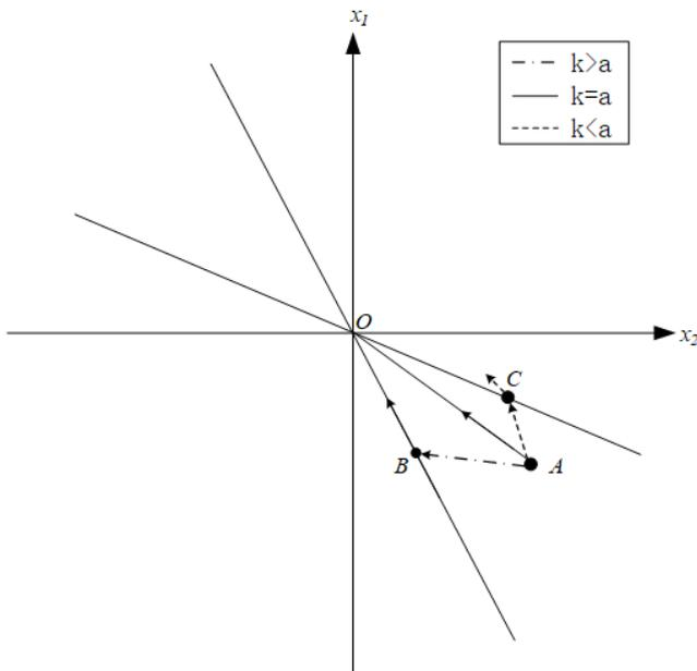
Fig.6. Phase trajectory of initial point in  $No.1_i$  subspace
