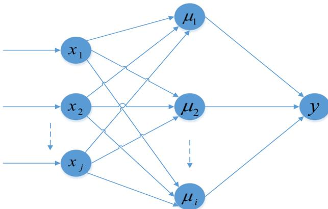
Fig. 2. RBF neural network flow diagram
