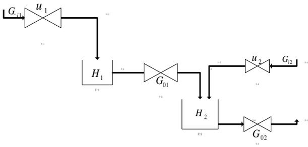
Fig. 1. Double tank liquid level control system.
