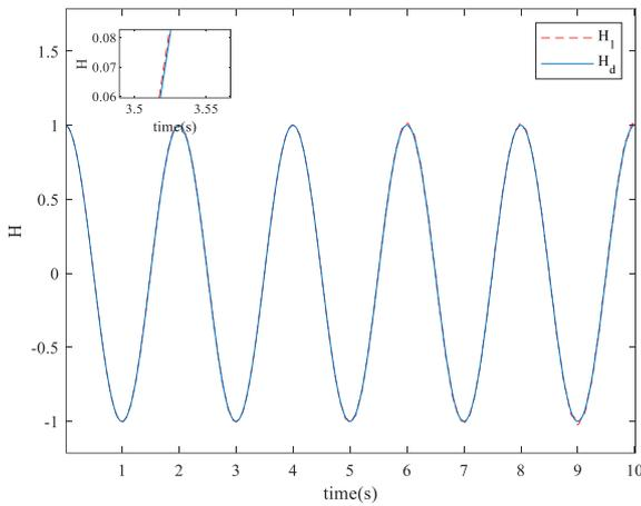
Fig.3. Trajectories of liquid level  $H_1$ , ideal position  $H_d$ .
