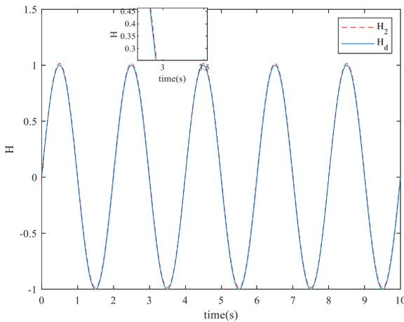
Fig.4. Trajectories of liquid level  $H_2$ , ideal position  $H_d$ .
