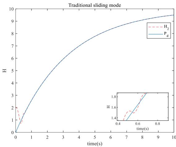
Fig.8. Trajectories of liquid level  $H_2$ , ideal position  $P_d$ .
