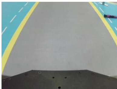
Fig.10. This picture is the original photo collected by the camera of the deep learning unmanned vehicle. It can be seen that the photo is greatly affected by the ambient light. In the process of unmanned driving, the ambient light is one of the factors most likely to affect the driving quality.
