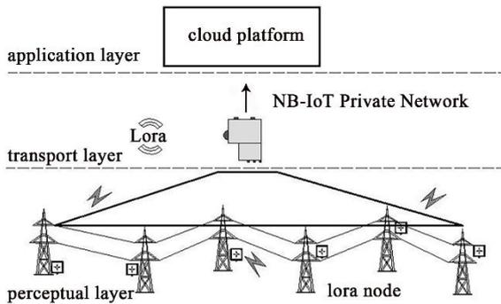
Fig. 1 Tower cloud platform monitoring system model
