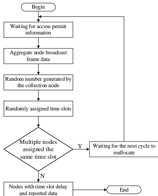
Fig. 3 Anti-collision algorithm flow chart
