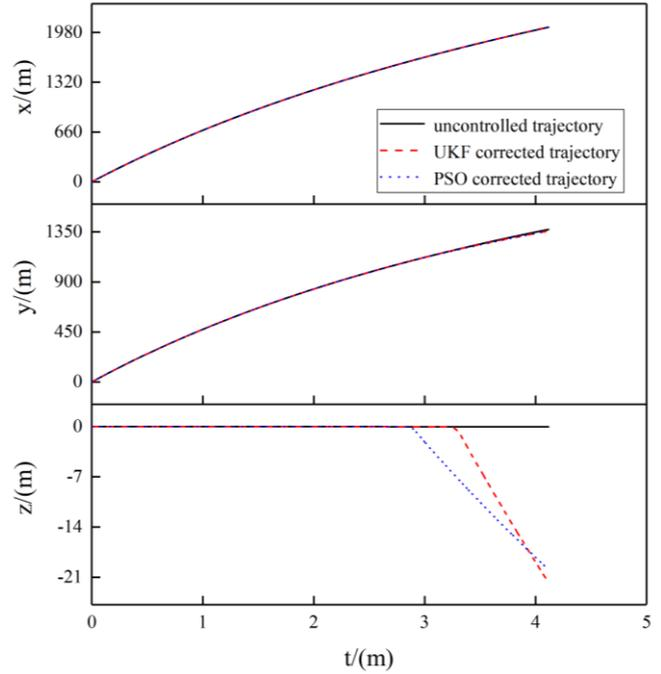
Fig.7. Trajectory curve at firing angle of 35 deg
