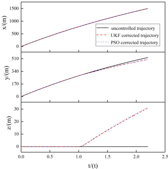
Fig.6. Trajectory curve at firing angle of 20 deg
