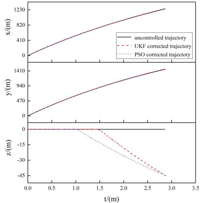
Fig.8. Trajectory curve at firing angle of 50 deg
