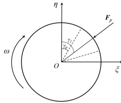
Fig.2. Schematic diagram of the action of the pulse force
