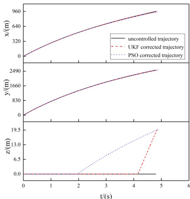
Fig.9. Trajectory curve at firing angle of 70 deg
