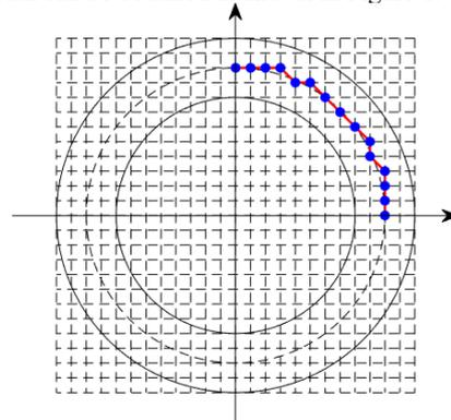
**Fig.1.** Trajectory diagram of Bresenham circle algorithm
