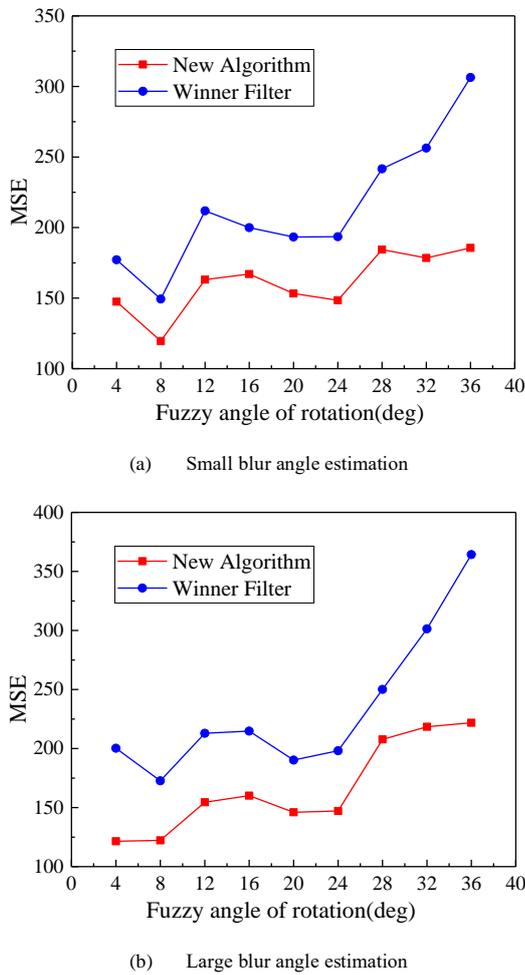
Fig.4. MSE values of two algorithms for estimation of different blur angles
