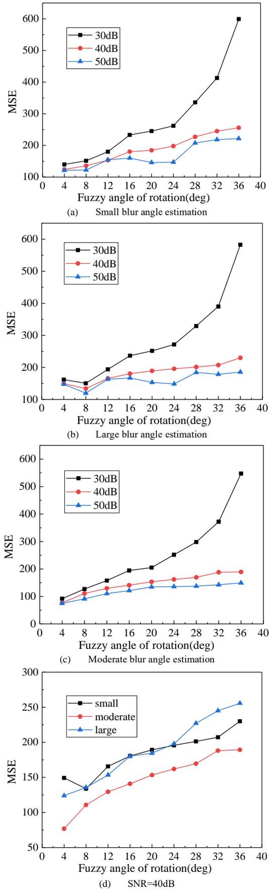
Fig.5. MSE values of image restoration under different blur angle estimation and noise conditions
