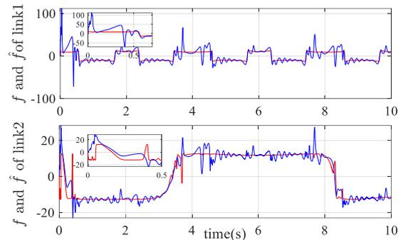
Fig. 6. Friction and compensation  $\theta(0) = 0$ .
