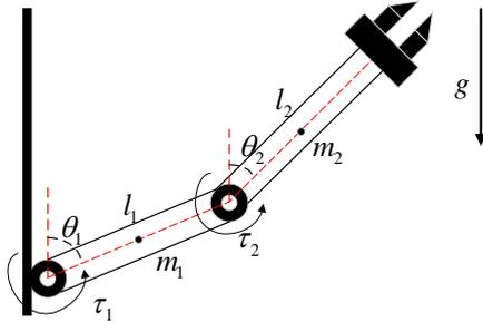
Fig. 2. 2-DOF robot manipulators Schematic Diagram.
