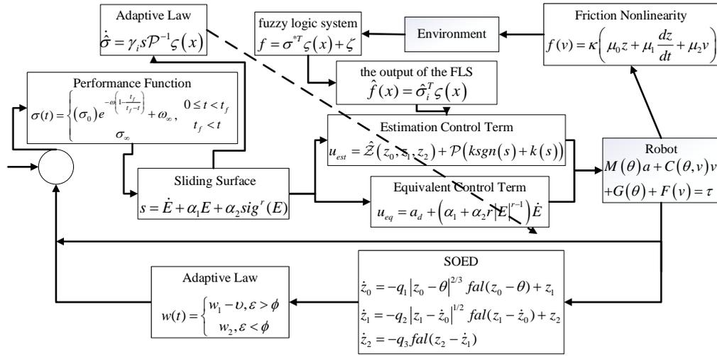
Fig. 1. Block diagram of the closed-loop system.
