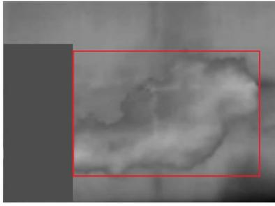
**Fig. 3.** OGI visualizes the gas into a grayscale image and labels the gas with a Faster R-CNN model for target detection.
