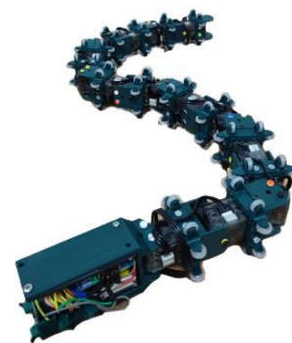
Fig. 1. A small serpentine robot and its joint module design.
