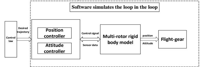
Fig. 4. Software in the loop simulation framework.
