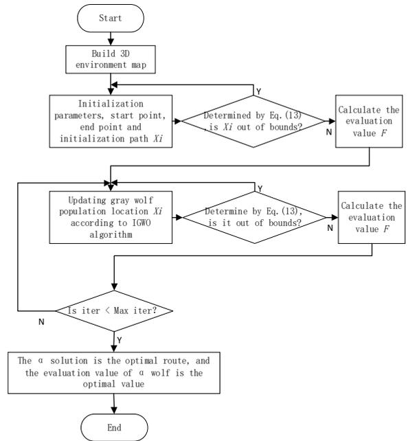
Fig. 5 Flow chart of UUV path planning based on IGWO
