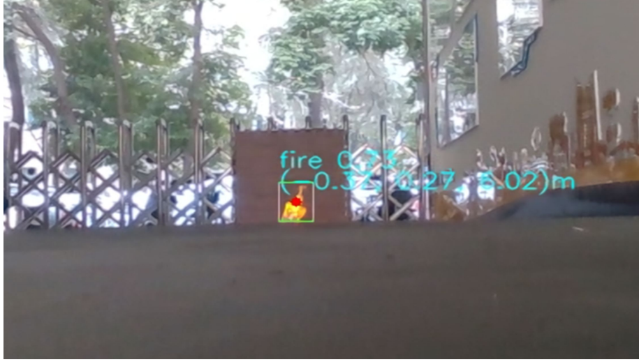
FIGURE 8 Flame Detection and Localization Results.
